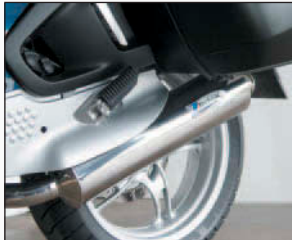
The Z4000 Exhaust allows sufficient clearance for mounting the stock saddlebags.
