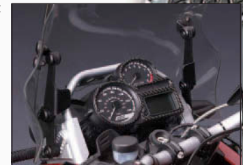
Z2243 articulating arm in its highest upward locked position.
