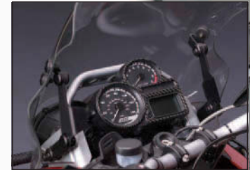
Z2243 articulating arm in its lowest downward locked position.
